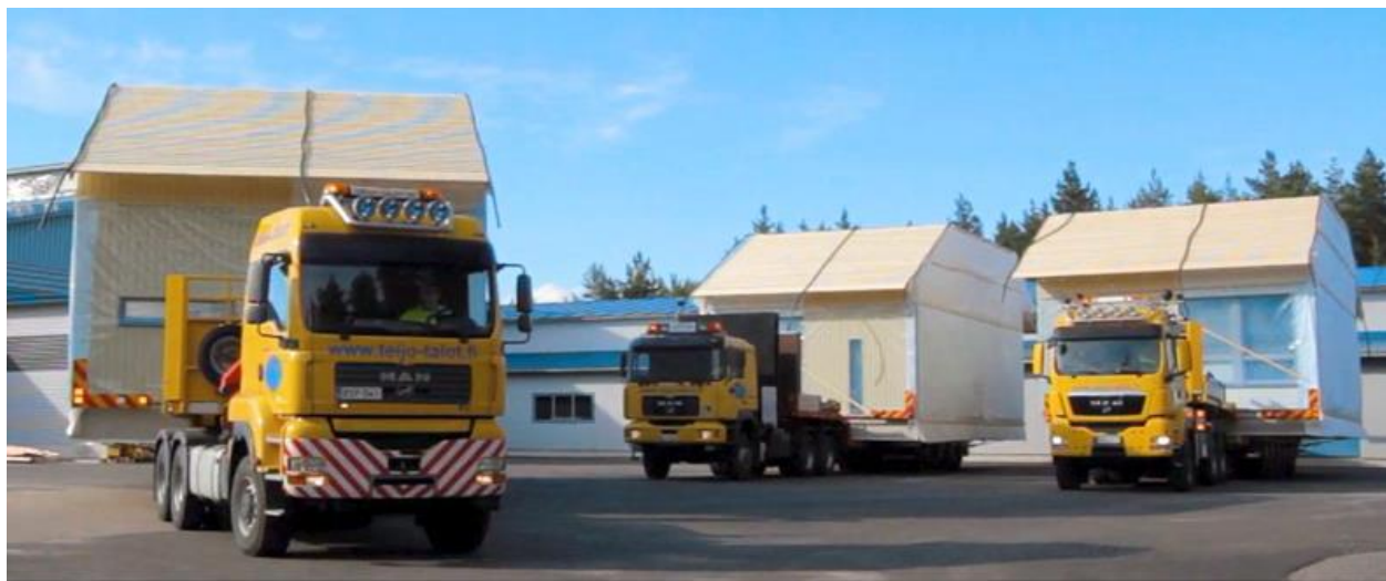
Figure 1. The Teijo-talot modules are transported with the foundation attached. Photo: www.teijotalot.fi
