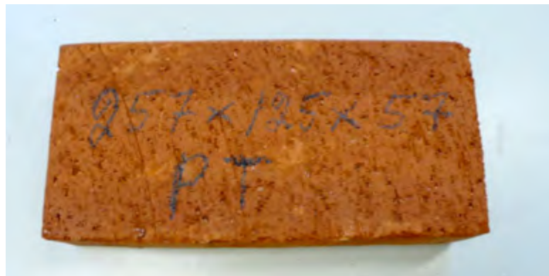
Figure 2.52. PT stands for 'peruskokoinen täystili', i.e. standard size solid brick of the dimensions 257 x 123 x 57 mm according to the producer (Wienerberger).
