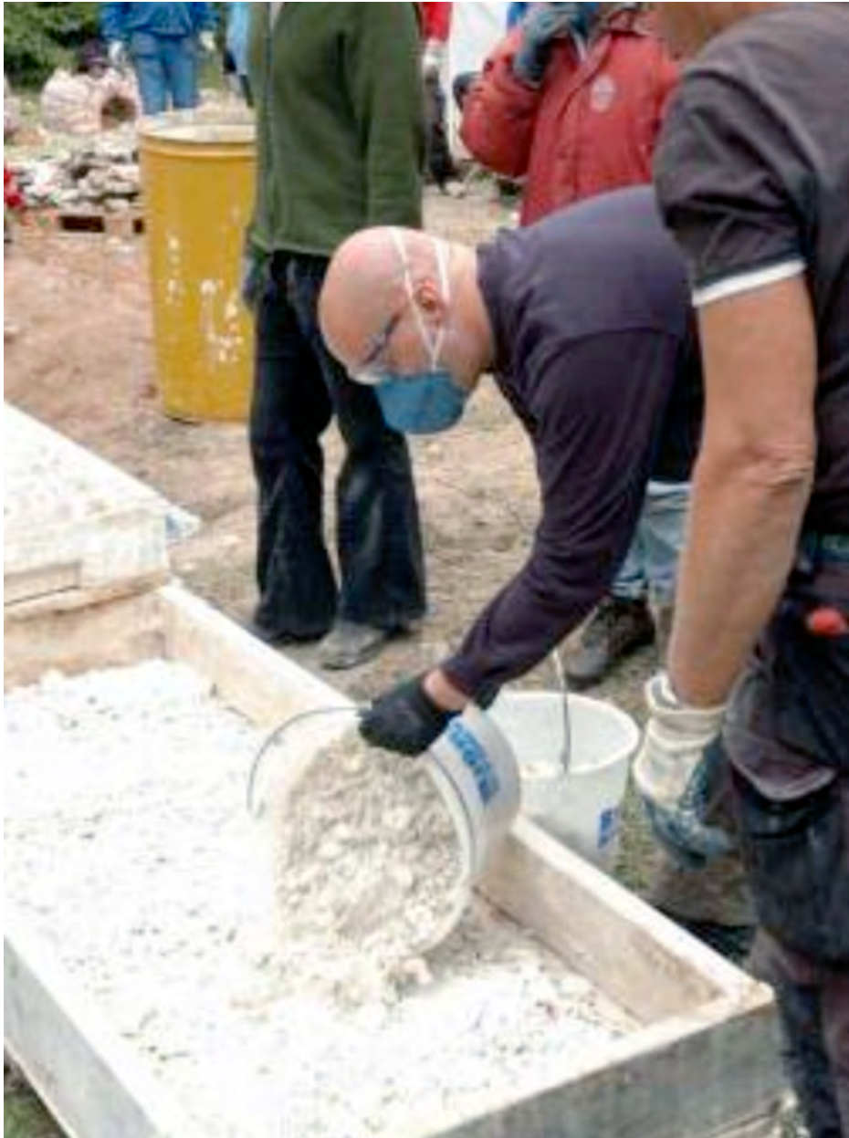
Figure 7. Sorting out the completely burned lime stone.
