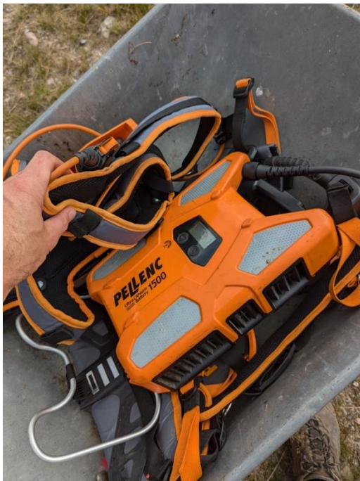
Picture 5: Pellenc ULiB 1500 with harness. Fills an entire wheelbarrow. A lot more energy than we would need for this project, but using it avoided downtime at a very busy time of the year and was a real eye opener to the potential work one could do with this system. Picture Credit: Joshua Finch, Novia UAS
