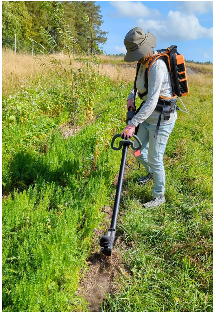
Picture 6: Pellenc Cultivion with ULiB 1500 in action edging a tree line; note the soil scattering to the bottom of the image. Photo Credit: Joshua Finch, Novia UAS
