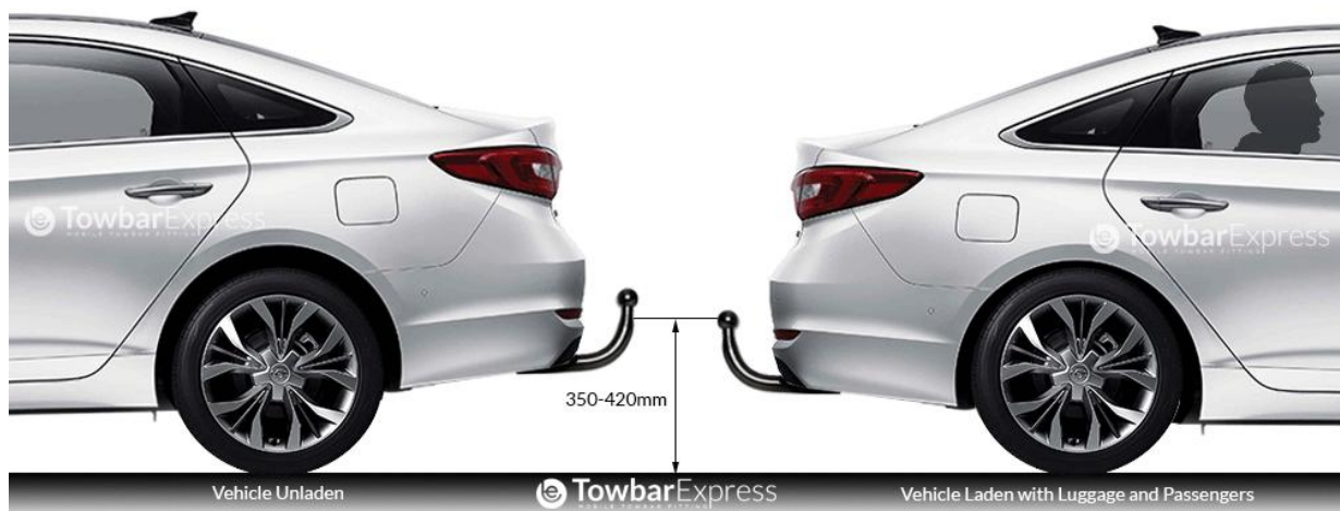
Figure 20: The tow bar height of a car when loaded Source: (Towbarexpress, 2017)
