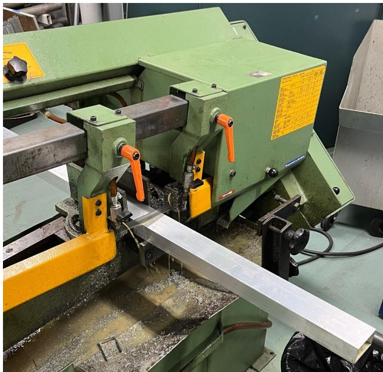
Figure 64: Cutting process of the aluminium profiles
