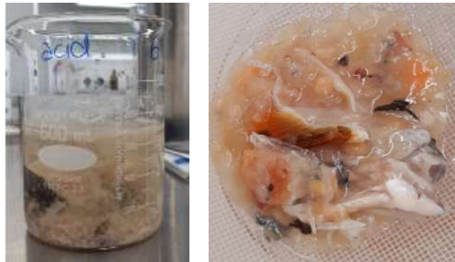
Figure 95: Solubilization and filtration of the fish waste.
