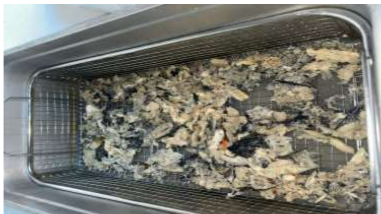
Figure 90: Fish waste after 6 hours in ultrasonic machine.
