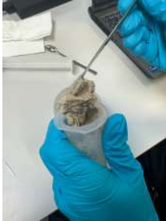
Figure 107: Inserting material in the syringe.
