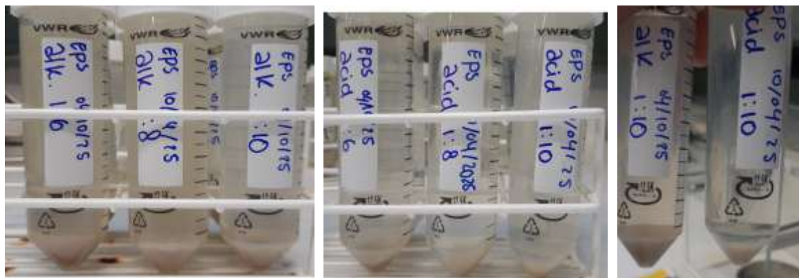
Figure 96: Alkaline and acidic solubilization comparison.
