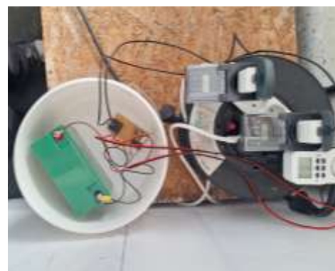
Figure 14: Battery and relay circuit picture
