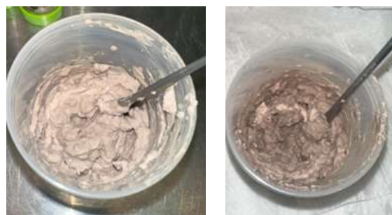
Figure 93: Paste with ultrasound (left) and paste without ultrasound (right).
