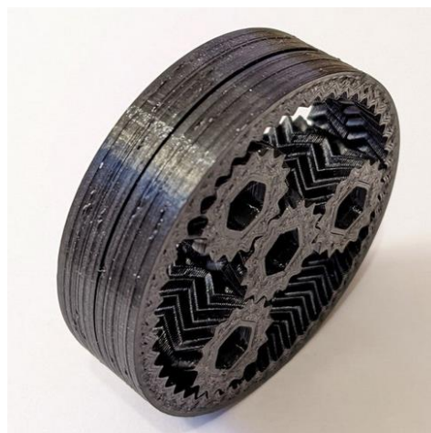
Figure 59: Split spline planetary gearbox.
