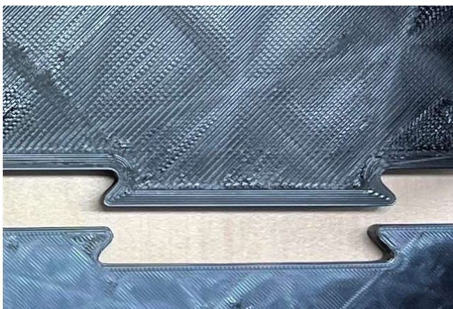
Figure 83. Case before assembly Detail of Dovetail. (own author).
