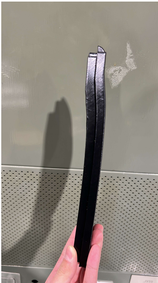
Figure 87. Failed Printing of Cover of Water Reservoir. (own author).
