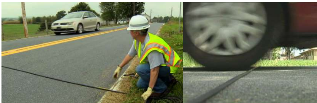
Figure 18- Image of pneumatic tube sensor working
