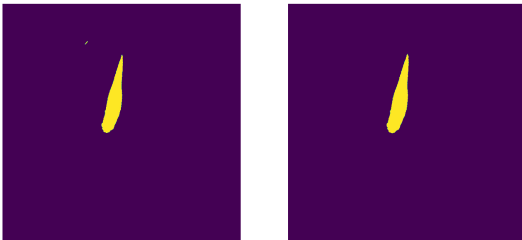
Figure 41. Binarized (left) and filtered by size (right) fish images
