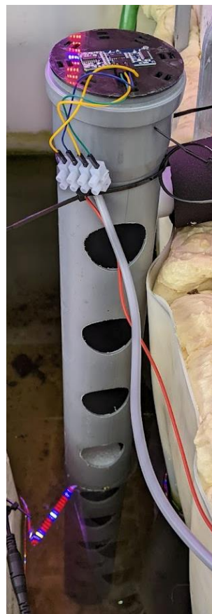
Figure 59. Water level sensor mounted
