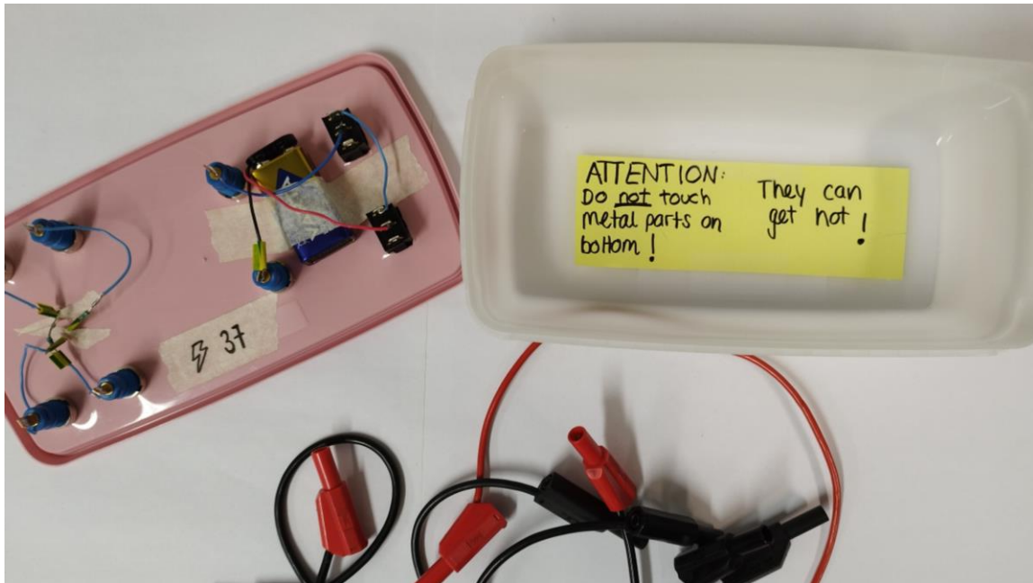
Figure 38 UV-circuit Box insides with Caution Sticker
