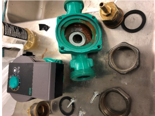
Figure 34 Corrosion on new pump
