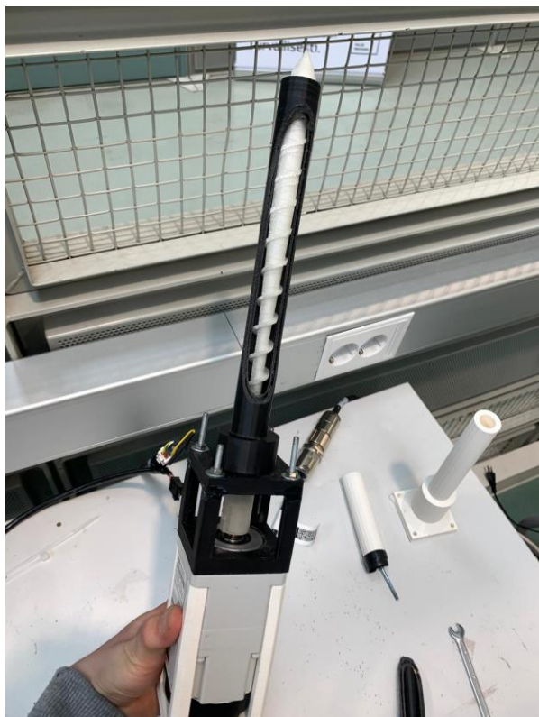
Figure 38: Screw inside the prototype extruder
