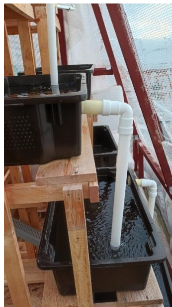
Figure 16: Testing of the system: DWC Racks
