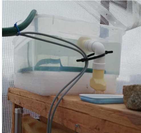
Figure 14: Testing of the system: tank that do not have an overflow system
