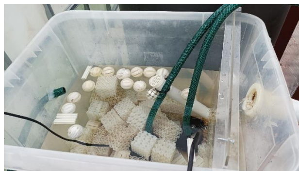
Figure 15: Testing of the system: bio filter
