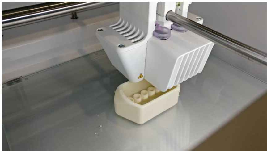
Figure 2.41 Nozzle printing process
