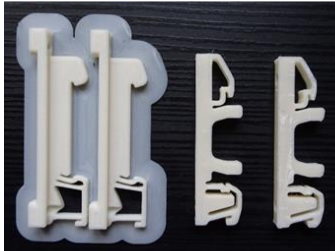
Figure 3.20 Mounting brackets for Raspberry Pi and circuit boards
