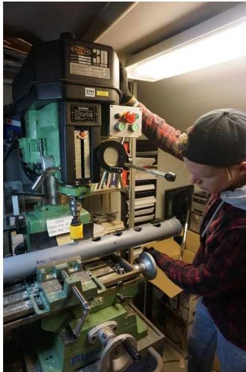
Figure 2.38 Drilling slots in vertical tower
