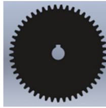
Figure 14 Fifty teeth gears
