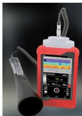
Figure 27 Ultrasonic meter (sonocheck).
