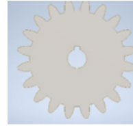
Figure 15 Twenty teeth gear
