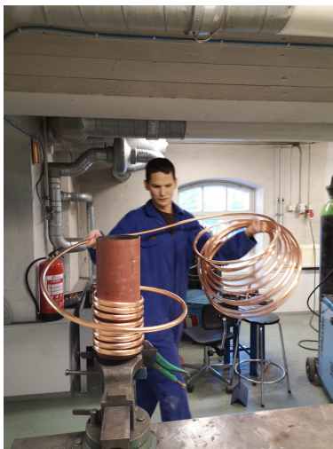
Figure 29: Construction progress of the spirals (own illustration, 2019)
