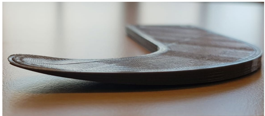
Figure 28: PLA part curling up during a print
