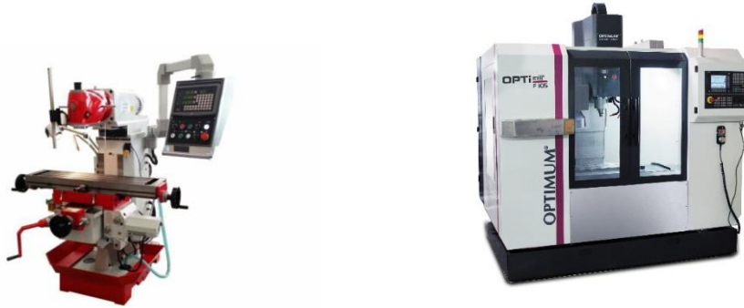
Figure 66: L: Manually milling machine; R: CNC milling machine
