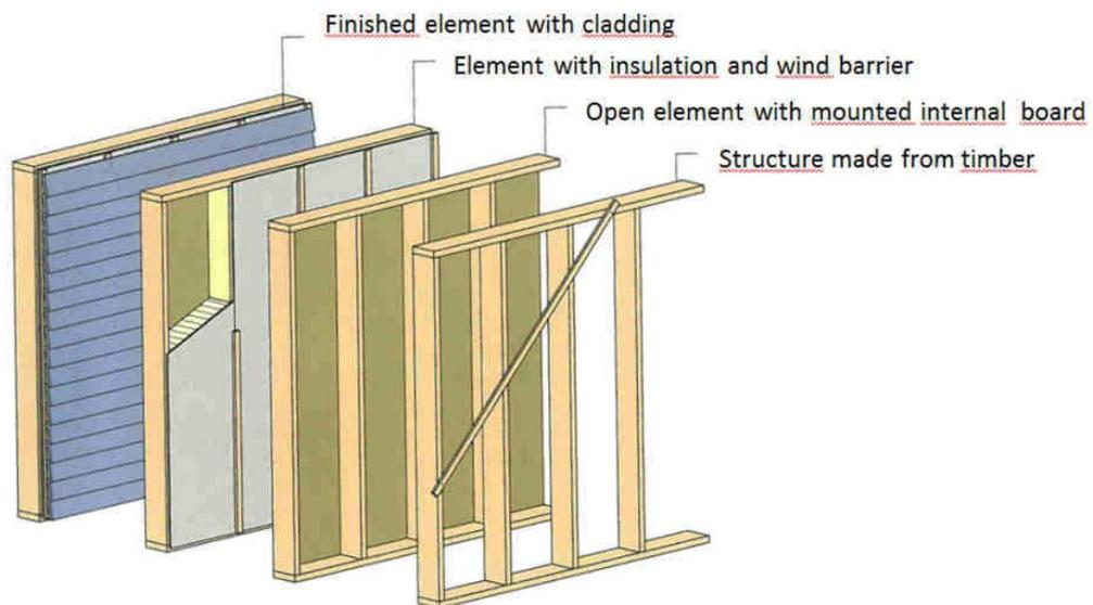
Figure 55 Construction of timber façade <sup>[17]</sup>
