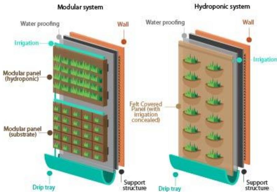
Figure 46 Two general types of green wall systems; modular and hydroponic [12]
