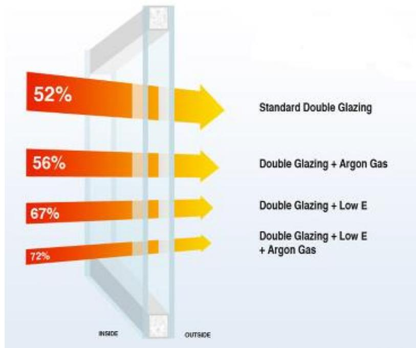
Figure 57 Heat loss reduction according to the method <sup>[30]</sup>
