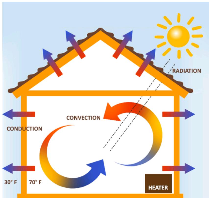
Figure 39 The idea of radiation, conduction and conversion <sup>[44]</sup>
