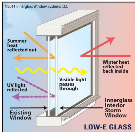
Figure 58 Low-e glass system (1) <sup>[31]</sup>
