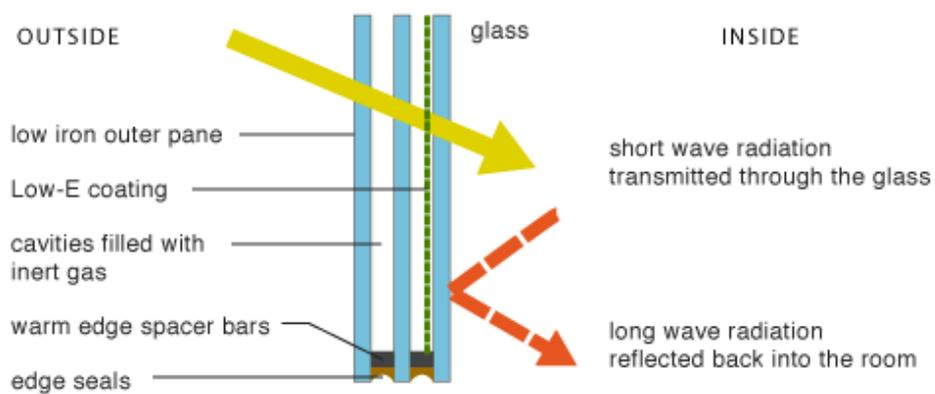
Figure 59 Low-e glass system (2) <sup>[32]</sup>
