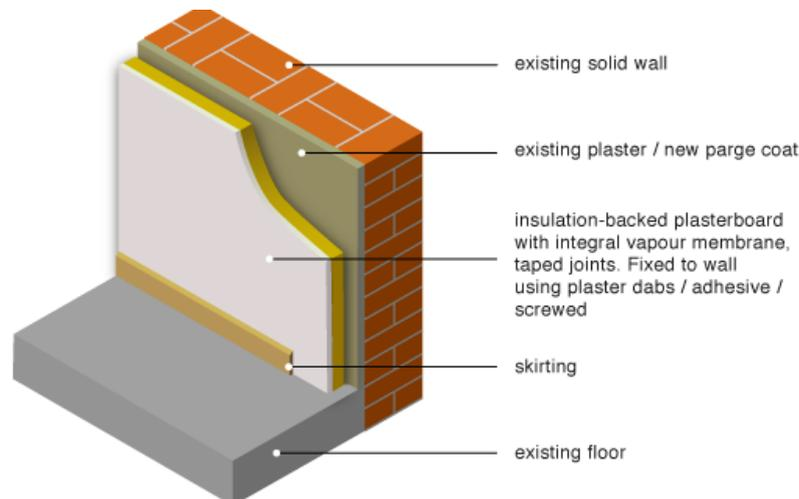
Figure 47 Plasterboard laminated fixed to the existing wall <sup>[13]</sup>
