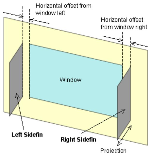
Figure 62 Local shading – sidefins <sup>[18]</sup>
