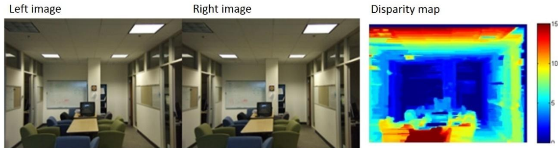
Figure 21 – Stereo vision depth estimation Source: https://se.mathworks.com/discovery/stereo-vision.html
