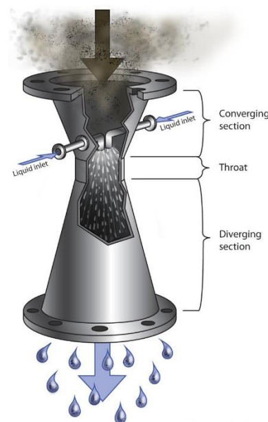
Figure 36 Venturi scrubber (Liewendahl, 2012)
