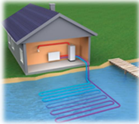
Figure 51: Water to water heat pump. Renova Retrofit 2015
