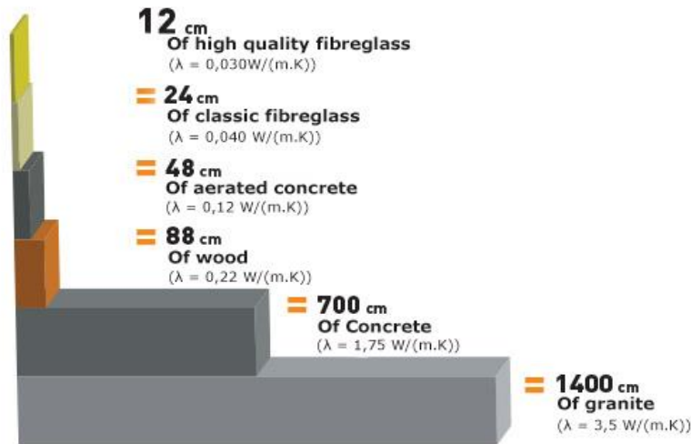
Figure 6: Equivalence between thickness and thermal resistance of different materials. MWNG. SA 2015
