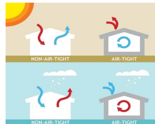
Figure 39: Comparison of air tight and non-air tight buildings
