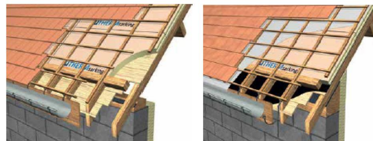
Figure 24: Lay without screen (Left) lay with screen roof underlayment and vapor barrier (Right). Utherm sarking on Unilin 2013
