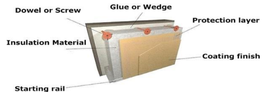
Figure 12: Wedge-Dowelled insulation "Loprobat 2011"
