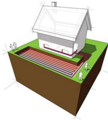
8.F. 2: Horizontal installation
